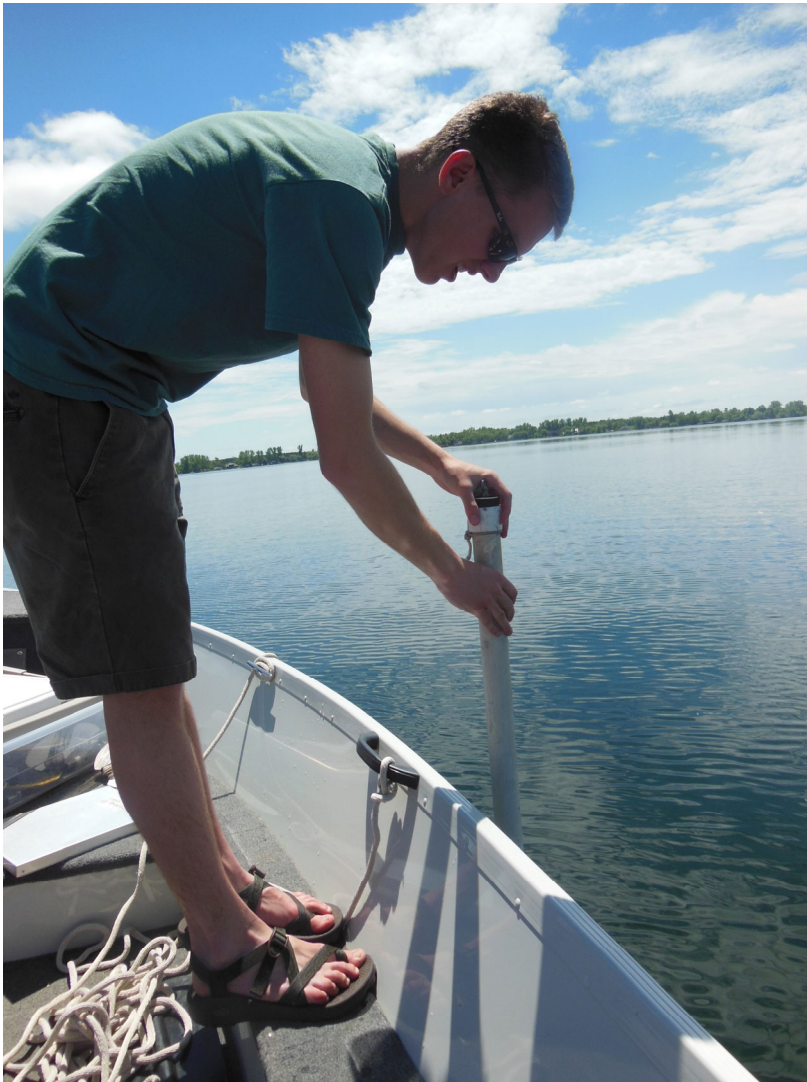
Matt Pawlowski, a 2013 Water Resources Intern with PRWD, uses a two meter integrated sampler to collect samples analyzed for chlorophyll-a, total phosphorus, and orthophosphate content on Lake Sallie.
